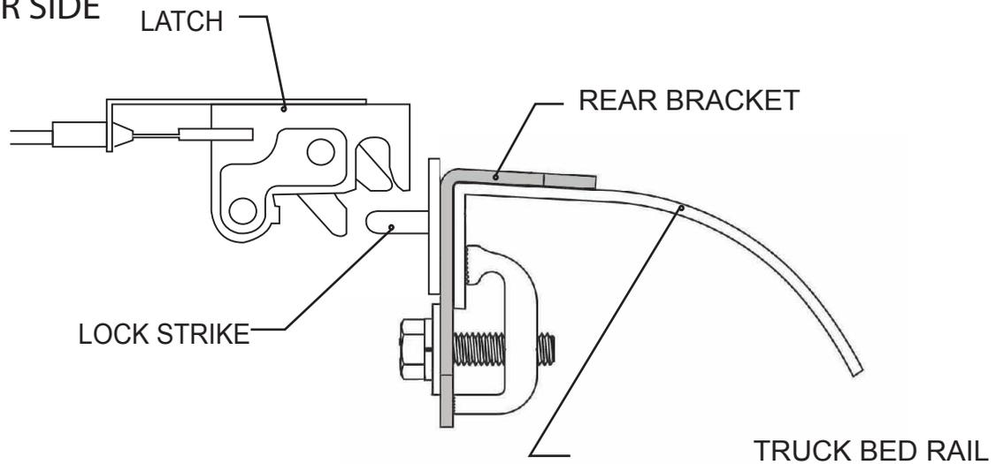
It may be necessary to adjust the latch side to side, to do so loosen the two latch mounting bolts, adjust latch and tighten.
